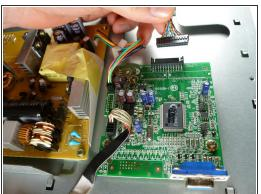
Remove the display cable located at the top of the circuit board by pulling it out towards the top of the monitor.
