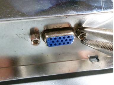
Using a nut driver (or if necessary, needle-nose pliers), remove the two nuts on either side of the VGA input.
