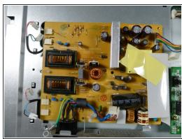
• With the needle-nose pliers, remove the four display connectors by pulling directly left.
