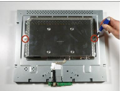
Remove the two 5.7 mm Phillips #2 screws located on either side of the EMI shield.
