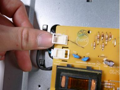
Remove the four little white clips located underneath the pieces of tape by lifting up on their left side.
