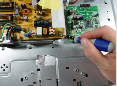
Remove the three gold 7.5 mm Phillips #2 screws and one silver 8.3 mm Phillips #2 screw from the power supply.
