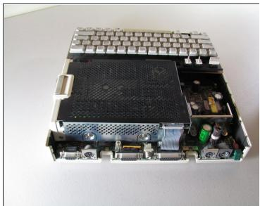
• Lift the handle straight up to remove.
