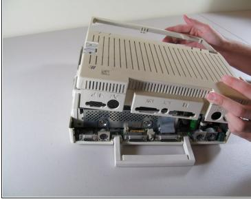
Slide the case toward the ports on the back, then grip under the catch and pull up while moving toward the ports to remove.
