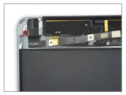
Remove the final 2.6 mm Phillips screw securing the headphone jack to the rear case.
