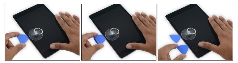
• Insert a second opening pick alongside the first and slide the pick down along the edge of the iPad, releasing the adhesive as you go.
