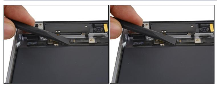
• Use the flat end of a spudger to flip up the retaining flap on the left antenna ribbon cable ZIF connector.
