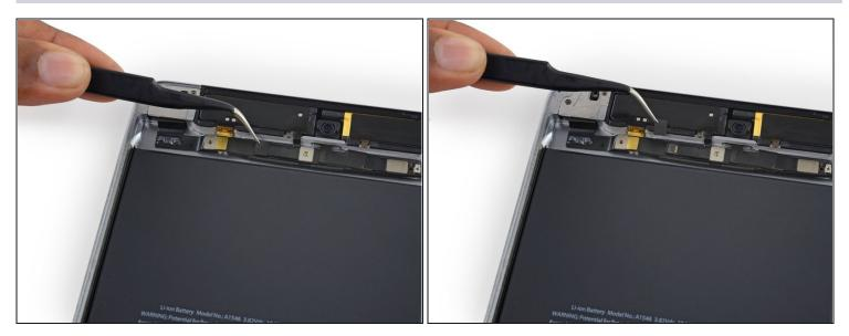
• Use <u>tweezers</u> to remove the small piece of tape covering the the left antenna ribbon cable ZIF connector.
