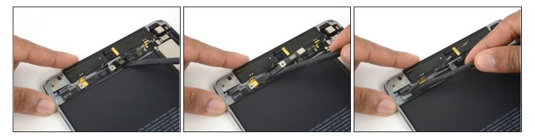
• Slide the flat end of a spudger under the headphone jack ribbon cable to separate it from the adhesive holding it to the rear case.
