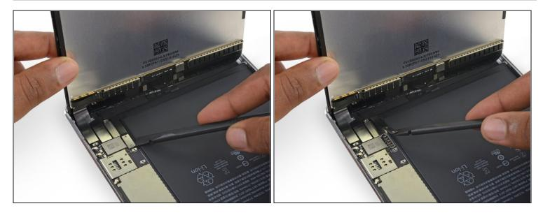
A When disconnecting any press connectors from the logic board, be sure to lift the connector straight up to avoid ripping the socket off the board.
