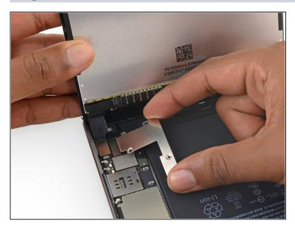
• Remove the battery/display cable bracket.
