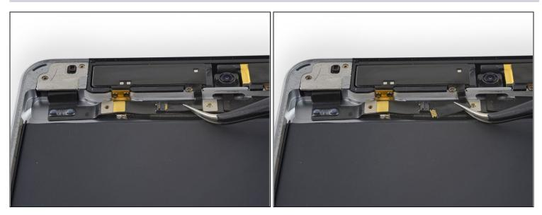
• Use tweezers to pull the antenna ribbon cable from its ZIF socket on the headphone jack ribbon cable.
