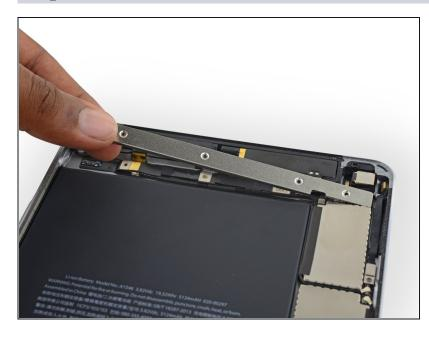
• Remove the upper component cable bracket.
