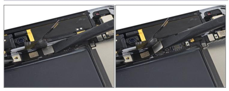
• Use the flat end of a spudger to lift the headphone jack cable connector from its socket on the logic board.
