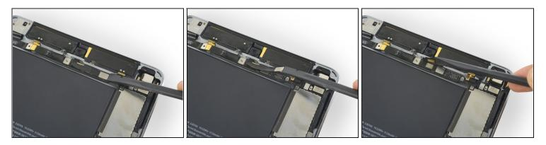
• Use the flat end of a spudger to disconnect the front camera press connector from its socket on the logic board.
