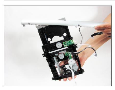
• Tilt the tray sideways and then pull back gently to separate the tray from the front panel.
