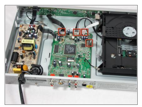
• Detach all the ribbon wires (4) attached to the motherboard
