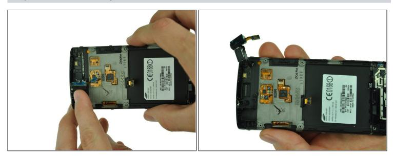
• Gently pull up on the audio jack, taking the attached ribbon cable with it.
