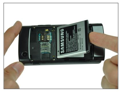
• Place your finger on the bottom of the battery and lift to remove.
