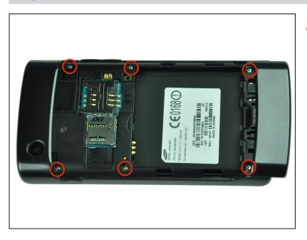
Remove the six 4.5mm #000 Phillips screws.
