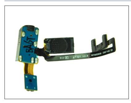
• The earpiece is attached to the 3.5mm audio jack. You will need to replace the entire assembly.
