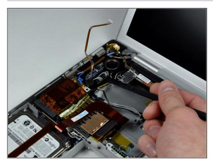
Disconnect the large gray and black battery connector cable from the left I/O board.
