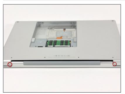
Rotate the computer 90 degrees and remove the two 3.2 mm
