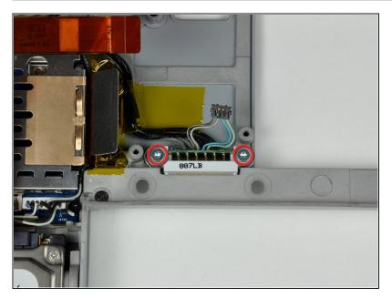
Remove the two silver T6 Torx screws securing the battery connector to the lower case.
