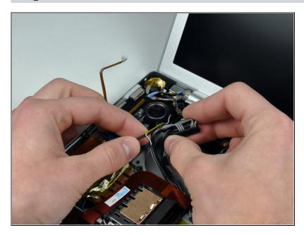
Thread the gray and black power cable beneath the speaker cable, and lift the battery connector out of the computer.
