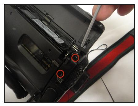
Remove the two top screws from the microphone.
