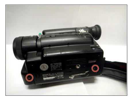
Use a Phillips #00 screwdriver to remove three screws: one from the bottom, one from the side, and one from the top of the camera.
