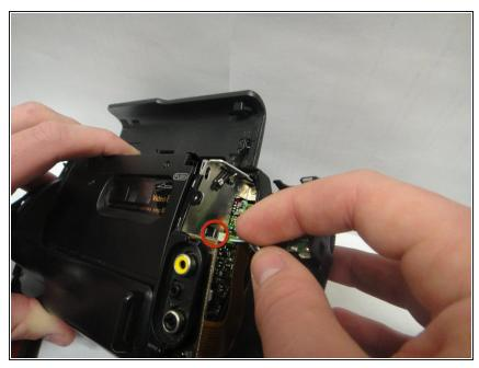
Carefully remove the electrical connector from the circuit board.
