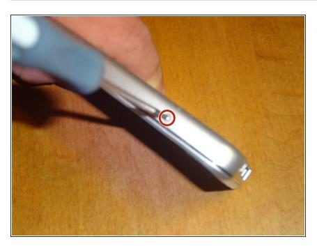
Remove 1 screw from the lower left side of the device.
