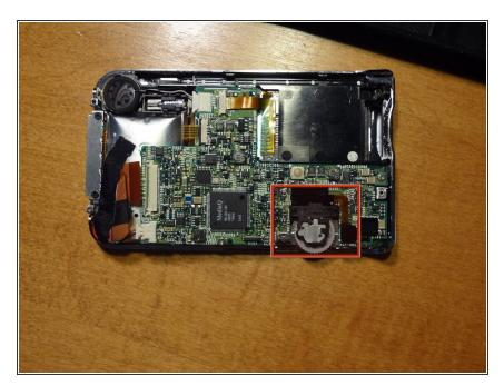
Locate thumb dial on top right side of the board.
