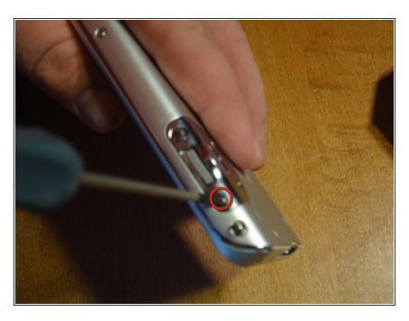
Remove the screw from thumb dial panel on the right handed side of the device.
