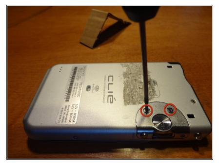
First, place the device with the screen side facing down. Remove the 2 screws from the thumb dial panel located on the upper right hand side.
