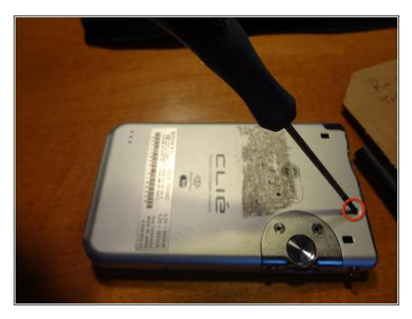
Remove the screw directly above the thumb dial panel.
