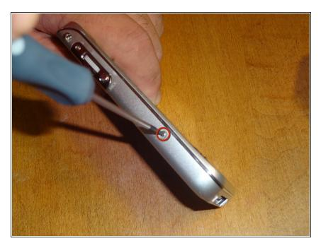
Remove screw from lower right side of the device.
