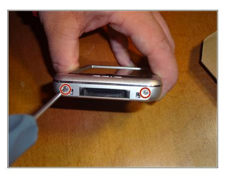
On the bottom of the device, remove both the left and right screws.
