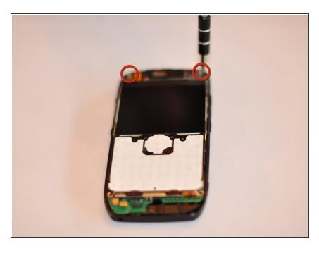
Using Torx number 4 unscrew the two 0.7 mm screws at the top of the device.
