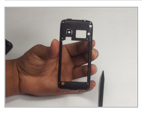
Replace the secondary rear panel which has the camera lens attached.
