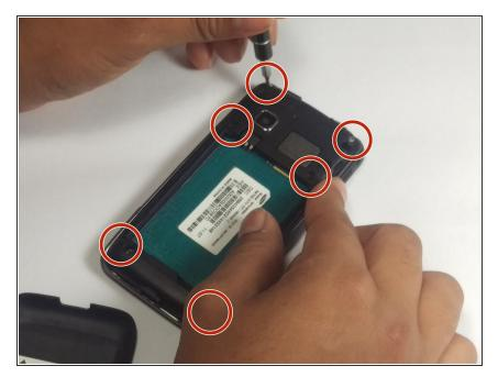
Remove the (6) 4mm screws using a Phillips #00 screwdriver.
