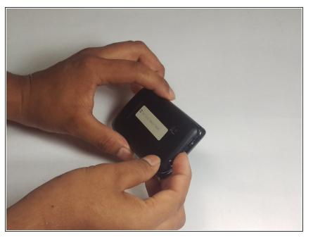
Using your hands, carefully remove the back panel by popping the open slit, near the headphone jack, outwards.
