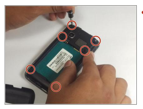
Remove the (6) 4mm screws using a Phillips #00 screwdriver.
