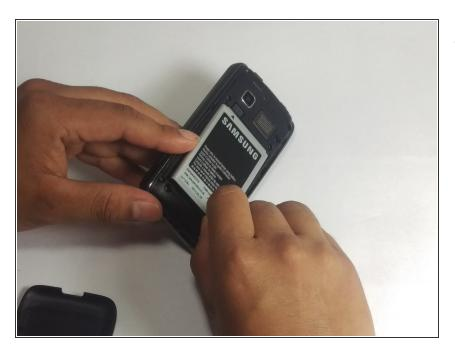
Using your fingernail or nylon spudger, remove the battery by lifting upward in the recess of the bottom right corner.
