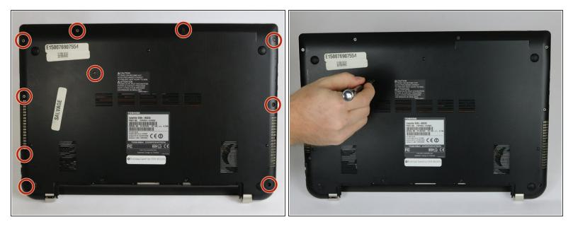
Remove the ten 7 mm Phillips #1 screws that secure the back cover.
