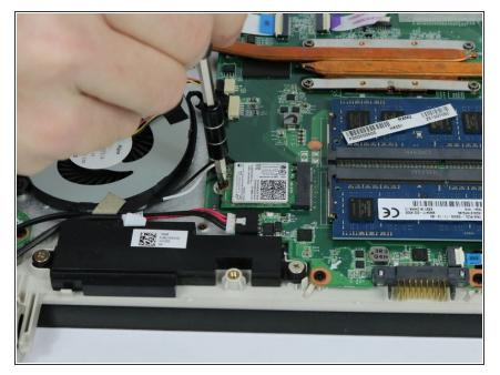
Remove the single 4 mm Phillips #1 screw holding the Wi-Fi adapter in place.
