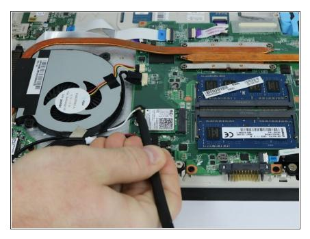
Using the pointed end of the Spudger, gently disconnect the antenna (white and black wires) from the Wi-Fi adapter.
