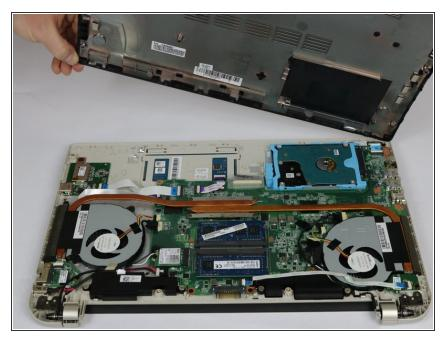
• Once all retaining tabs are released from the frame, you can pull up on the back cover to remove it.
