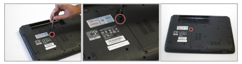
• Use the Phillips #1 screwdriver to remove the 6.5mm Phillips #1 screw.
