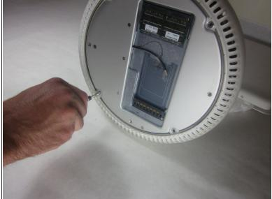
Remove the four 25mm T-15 screws.
