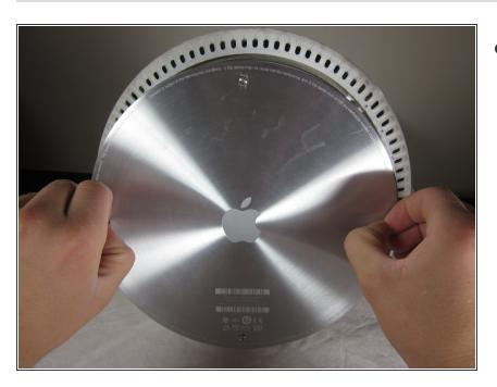
Carefully remove the base access panel.
