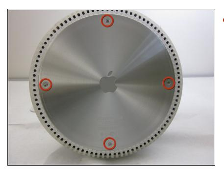
Loosen the four Phillips #0 screws.
