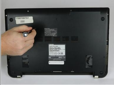
Remove the ten 7 mm Phillips #1 screws that secure the back cover.
