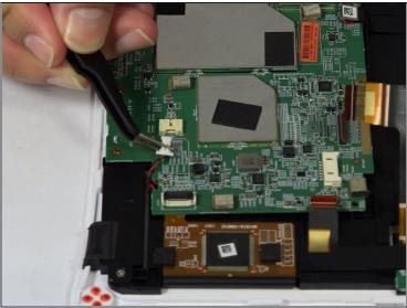
• Disconnect the Right speaker by grabbing the wire head by its sides and pulling it back from the connector.
