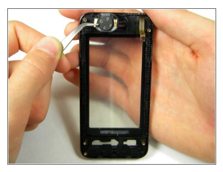
Using tweezers to grasp the pins of the speaker, gently lift the speaker up out of its setting in the front case.
