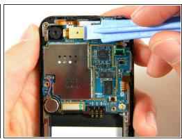
Use the plastic opener tool to detach the three ribbons on the motherboard.
