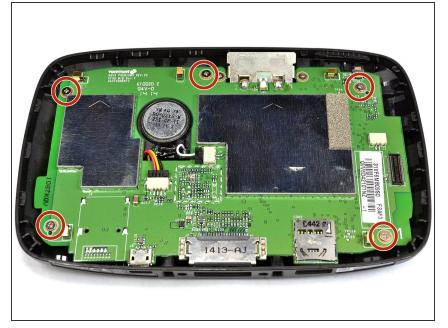
Unscrew the five 4mm screws using the Phillips #0 screwdriver.
