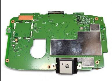
Remove the motherboard from the casing.
