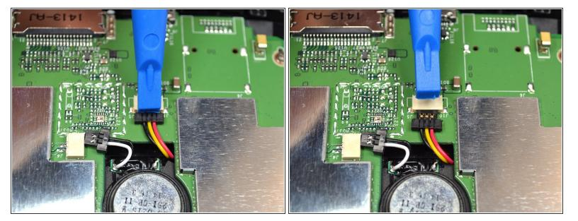
Unplug the second connector using the plastic opening tool.
