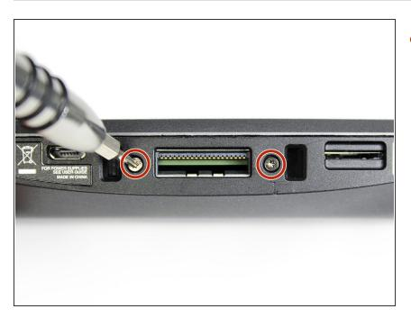
Unscrew the two 3mm screws at the base of the device using the Torx T5 screwdriver.
