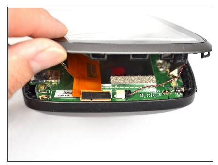
With the screen casing unlatched, locate the right side where the two connectors are.
