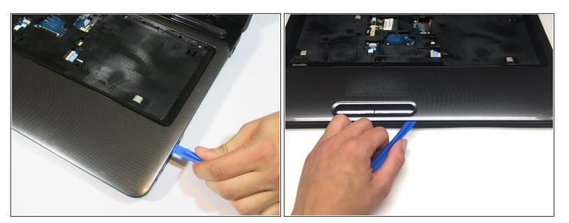
Pry under the top case housing along the perimeter with a plastic opening tool.
