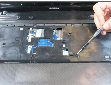
Remove five 5mm screws with the screwdriver.
