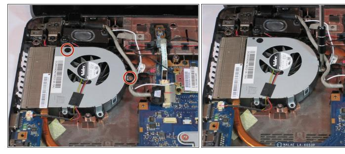
Remove the two 5mm screws using screwdriver.
