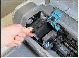
• Lift both of the teal plastic covers located on top of the cartridges. Next, grab the ledge located on the top of the cartridges, and gently lift both cartridges out of the printer.
