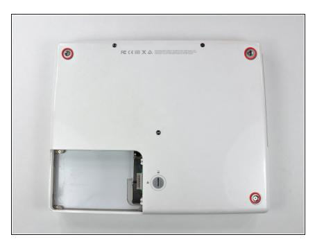
Remove the three newly-revealed Phillips screws.
