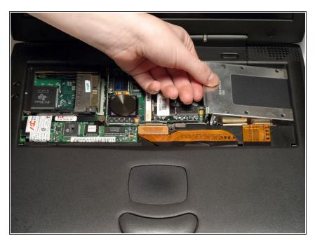
• Grasp the hard drive bracket on the left side and pull up and to the left.
