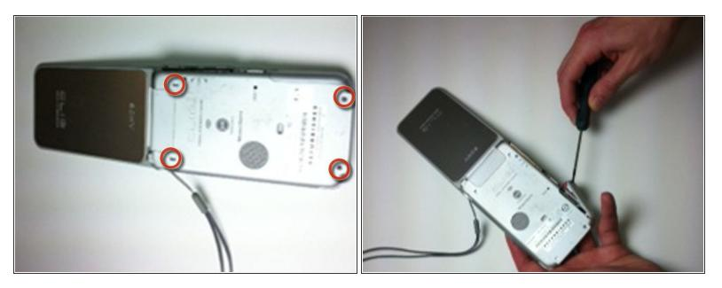
Use a #00 Phillips screwdriver to remove screws on the back plate and the side of the device.
