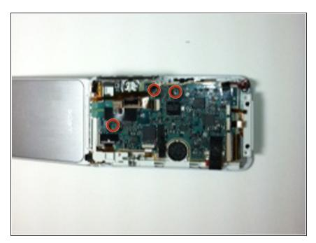
Use the #00 Phillips screwdriver to loosen and remove the screws on the motherboard.
