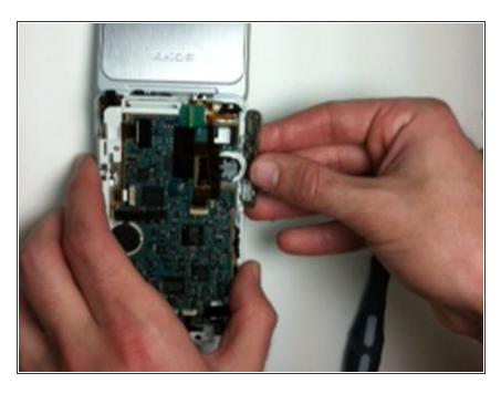
Remove the volume rocker from the side panel of the device.
