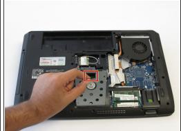
• Use the black tab to pull the hard drive up and out of the laptop.
