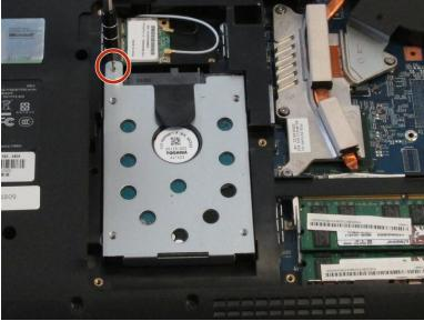
• Use the Phillips #1 screwdriver to remove the 3.5mm Phillips #1 screw.
