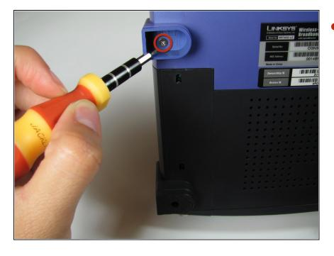
Use a Phillips #2 Screwdriver to remove the two 5.8 mm screws holding the front case to the motherboard.
