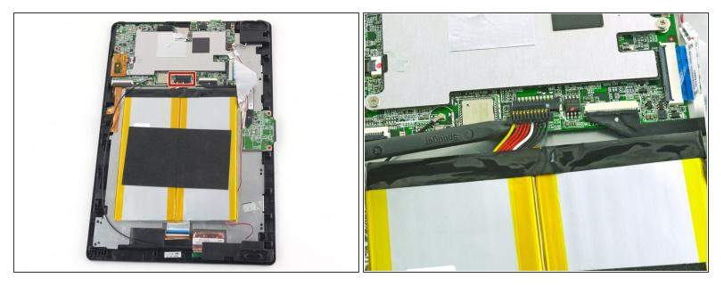
• Use a spudger to disconnect the black bundled cable connector from the motherboard.
