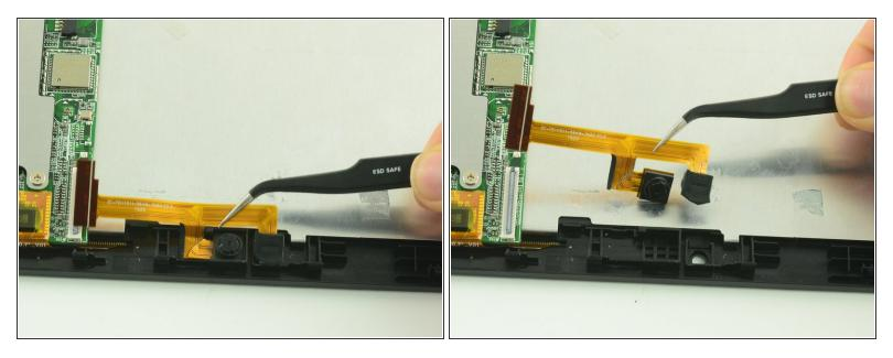
• Use tweezers to lift the camera assembly away from the device.
