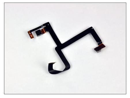
The DSi has two VGA CMOS digital cameras (0.3 megapixels); one on the internal hinge pointed towards the user and the other in the outer shell.
