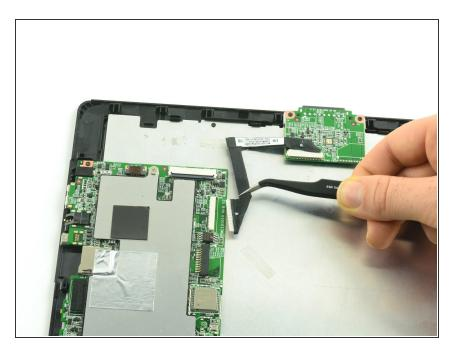
Use tweezers to pull the dock contact display cable away from the connector on the motherboard.
