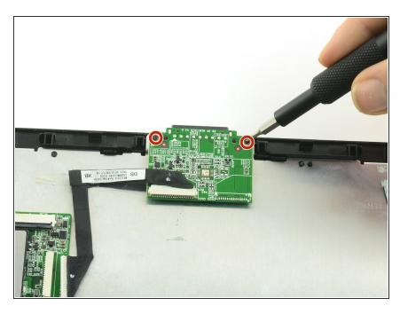
Use a Phillips #000 screwdriver to unscrew the two 4.2mm screws from the circuit board containing the dock contact.
