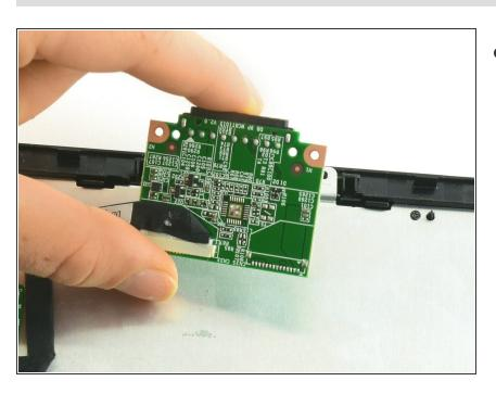
Lift the dock contact assembly away from the device.
