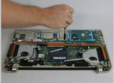
• Remove the four 4 mm Phillips #1 screws mounting the heat sink to the motherboard.
