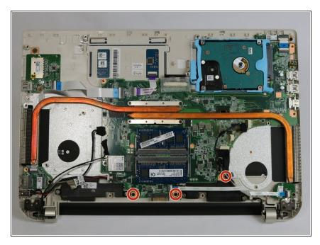
Remove the three 4 mm Phillips #1 screws holding the motherboard in place.
