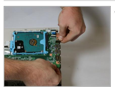
Lift on the motherboard from the USB port area while pulling the frame away from motherboard.
