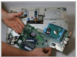
Once all connectors are separated from the motherboard and the USB port area is freed, carefully lift on either side of the motherboard to remove it.
