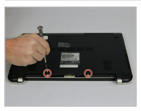
Remove the two 7 mm Phillips #1 screws that hold the battery in place.
