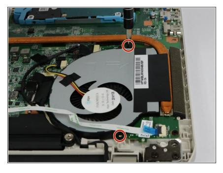
Remove the two 3.5 mm Phillips #1 screws that hold the cooling fan in place.
