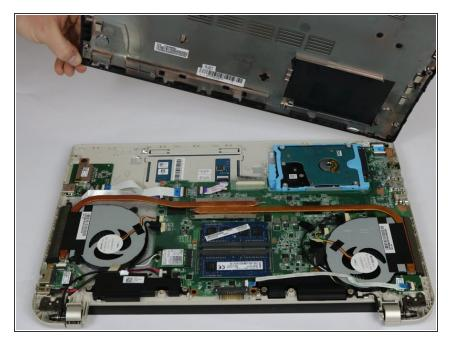
Once all retaining tabs are released from the frame, you can pull up on the back cover to remove it.
