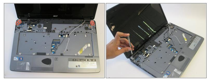
Use the Phillips #1 screwdriver to remove the four 11mm Phillips #1 screws.
