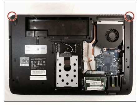
Use the Phillips #1 screwdriver to remove the two 6.5mm Phillips #1 screws.
