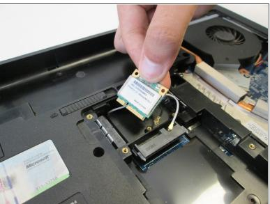
Remove the wireless module from the laptop.
