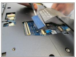
Lift the black latch upwards to release the ZIF connector.
