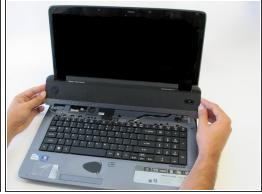
Gently hold the speaker panel by the sides and pull upwards to release the panel.
