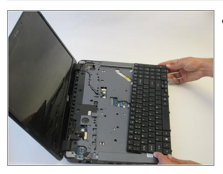
Remove the keyboard from the keyboard slot.
