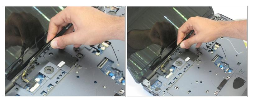
Release the cable from the tabs holding it in place.
