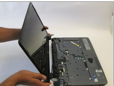
Grab the display assembly from the base and lift it up and off the base.
