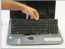
Insert a finger into the opening above the F11 key and pry the keyboard until it is released from the casing.
