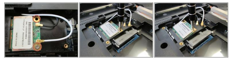
Use the Phillips #1 screwdriver to remove the two 4.8mm Phillips #1 screws.
