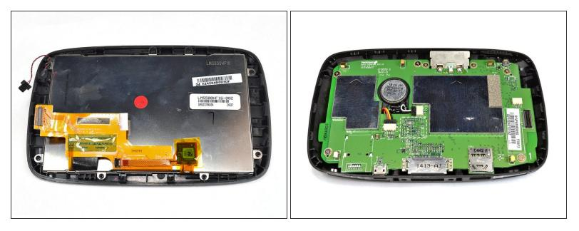
• Separate the screen casing from the motherboard casing.
