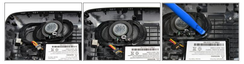
Insert the new speaker in the rubber grommet. Use the plastic opening tool to wrap the grommet over the speaker.
