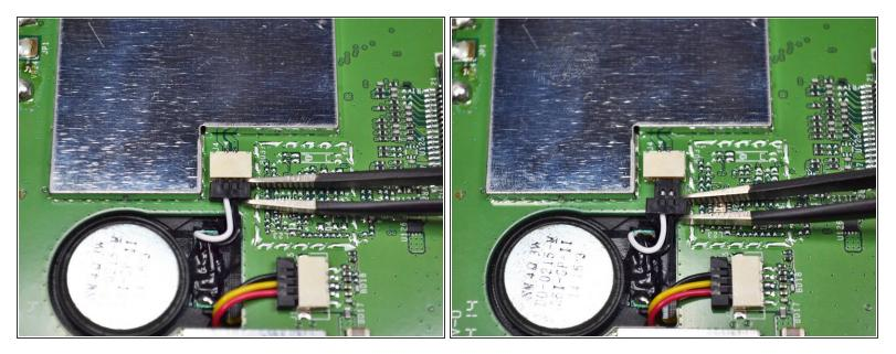
• Unplug the connector shown near the center of the motherboard using the tweezers.
