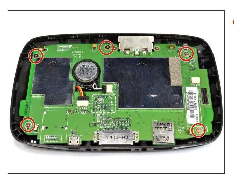
Unscrew the five 4mm screws using the Phillips #0 screwdriver.
