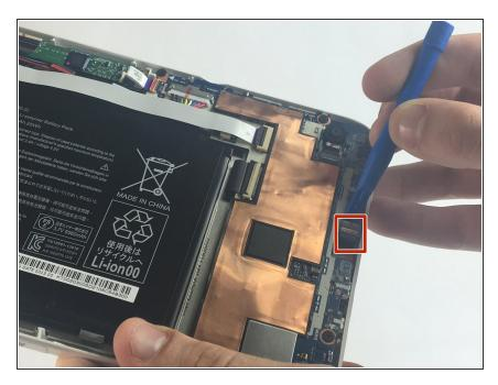
Loosen the retaining flap connected to the front-facing camera by lifting it with a plastic opening tool.
