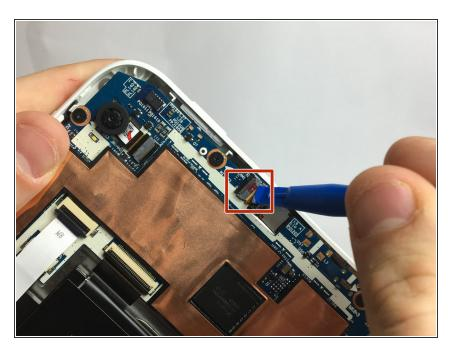
Remove the ribbon cord from its slot by pushing it out with a plastic opening tool.
