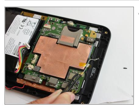
Disconnect the ground wire from the motherboard with tweezers.
