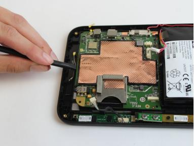
Pry off the clips that hold the motherboard down with the plastic spudger.
