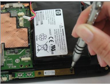
Remove the two 6mm Phillips screws with Phillips #0 screwdriver.
