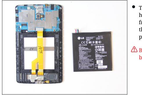
• There is a light adhesive holding the battery in the frame of the device. Gently pry the bottom the battery using a plastic pry tool.
