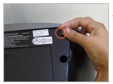
Peel off the two black square foams in front of the battery compartment to reveal a screw under each one.
