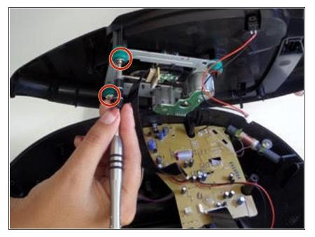
Using a Phillips #0, remove the two 11mm screws attached to the green legs underneath the top panel.
