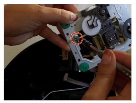
• Using a JIS 1, remove the 8mm screw on the grey, square plate.
