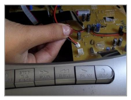
Unplug the red and black wires from the large yellow motherboard by pulling upwards.
