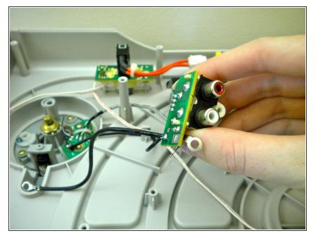
• Gently pull out the audio input jacks from the audio input housing.
