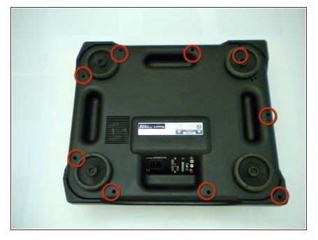
• Flip over the turntable and remove the nine screws on the outer edges.
