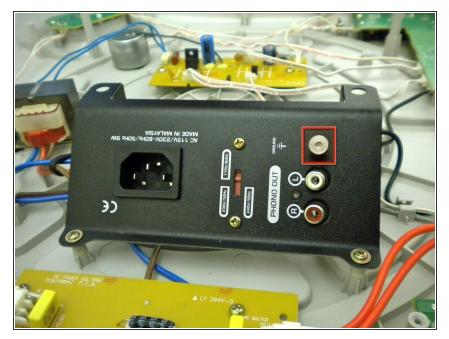
• Remove the grounding hardware located next to the audio jacks.
