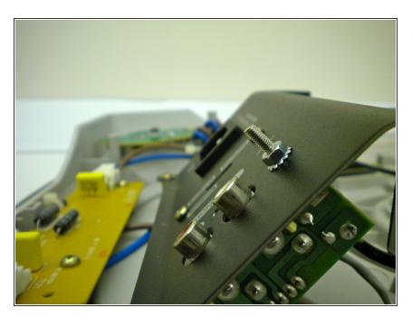
Remove the remaining nut and washer.
