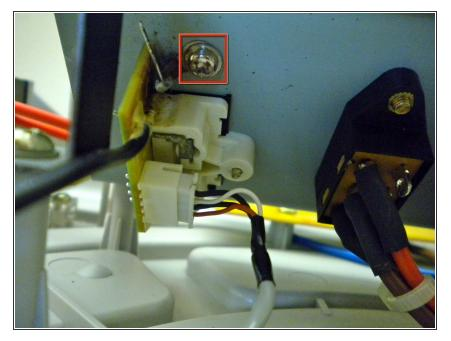
Remove the screw located on the back panel of the audio jack housing.
