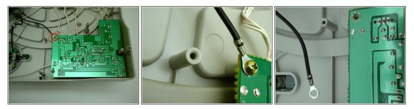
• Remove the screw that connects the audio jacks to the biggest circuit board via wire.
