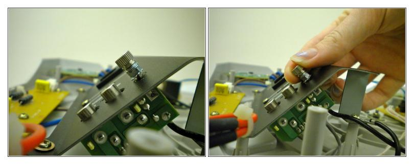
• Remove the ground screw and washers.
