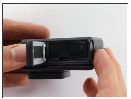
While pressing the button on the bottom of the GoPro, slide the battery door to the side to pop it open.
