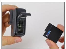
Grab the plastic flap on the battery and pull the battery out.
