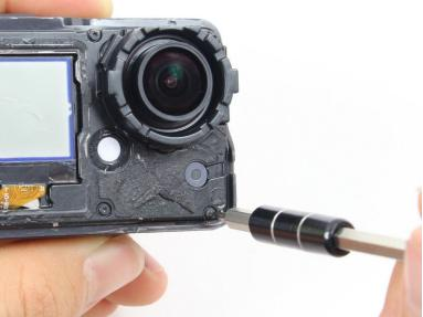
Remove the six T3 Torx screws.
