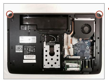
Use the Phillips #1 screwdriver to remove the two 6.5mm Phillips #1 screws.
