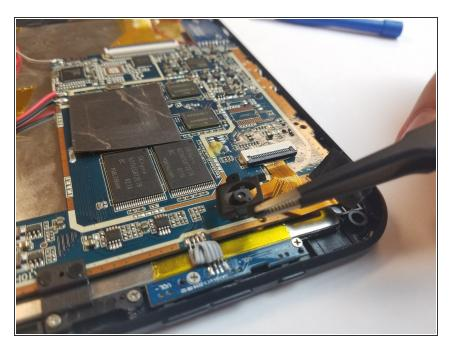
• Pull off the plastic camera cover with the tweezers so that the front-facing camera can move freely.
