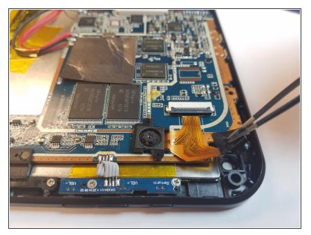
Pull the black tape away so that the rear-facing camera is no longer attached to the device.
