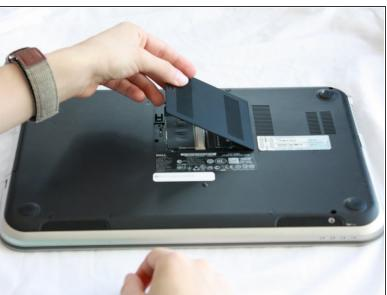
Lightly lift the RAM cover up and at an angle, away from the computer.
