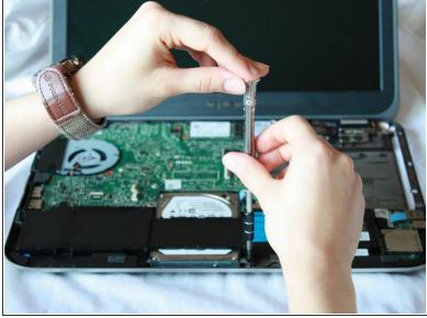
Use a J0 Bit screwdriver to remove the two 6 mm Phillips screws securing the battery located near the bottom of the laptop.
