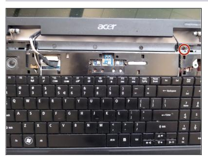
Remove the single screw next to the right hinge with a #00 Phillips Screwdriver.
