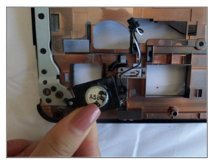
Remove the speaker carefully, extracting the wires from board.
