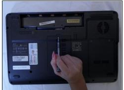
• Remove the fifteen screws from the back of the laptop with a Phillips #00 Screwdriver.
