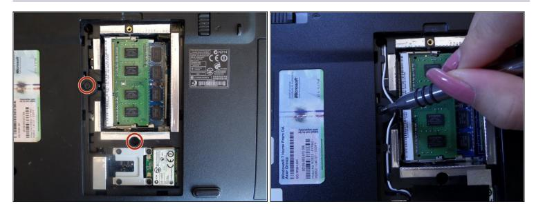
• Remove the two screws on the left and bottom of the circuit board with a #00 Phillips Screwdriver.
