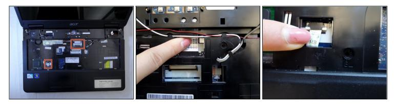
Disconnect the two blue and white ribbons by applying pressure downward and pushing them out of their sockets.
