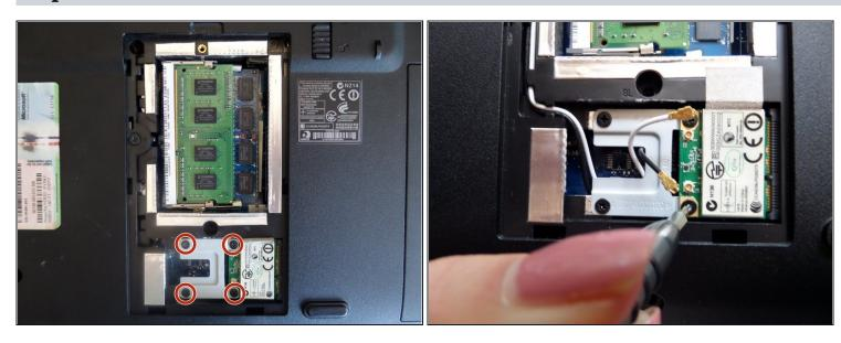
• Remove the four screws from the metal piece beneath the circuit with a Phillips #000 Screwdriver.
