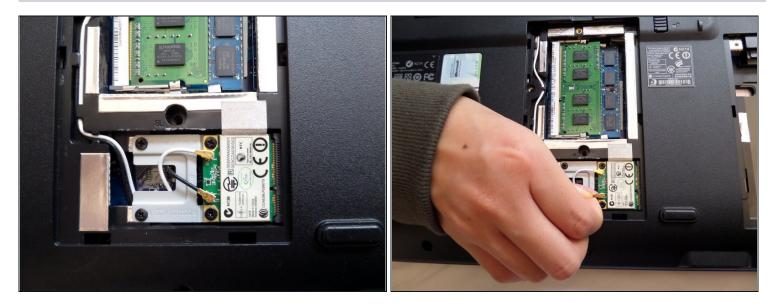
• Disconnect the black and white wires on the small circuit board by gently pulling them out of their sockets.
