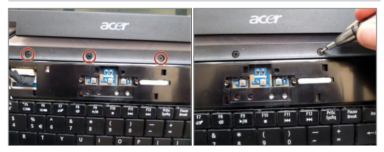
• Remove the three screws with a #00 Philips Screwdriver.
