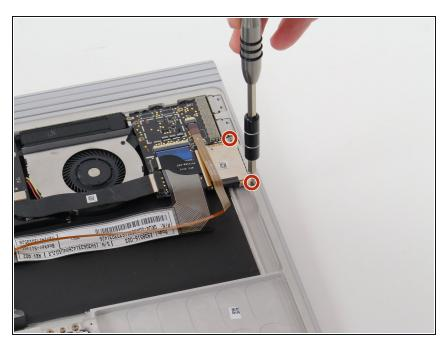
Use the T3 screwdriver to remove the two 4 mm screws on the right side of the SD Card Reader.
