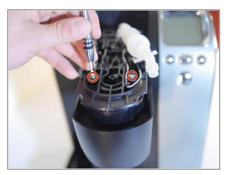
Remove the two 8mm screws with a PH #2 screwdriver.
