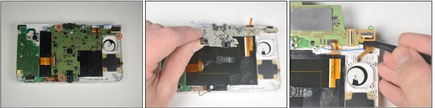
**⚠ Double check that all motherboard connection on the top of the board have been disconnected.**
