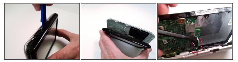
• Pry back cover off with a plastic opening tool just enough to see where the speaker is attached to the motherboard.
