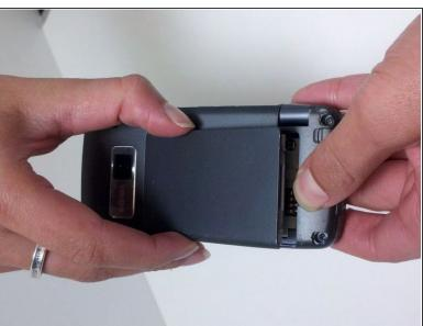
Remove the battery by pressing the button below it and lifting it out.
