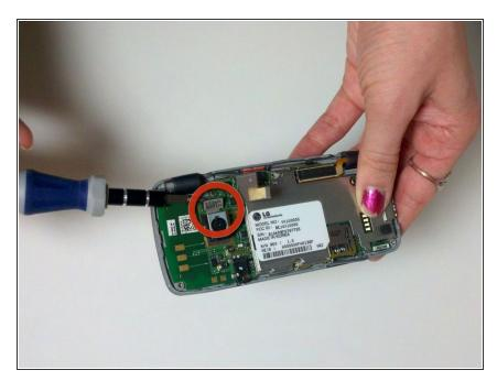
• Lift the connector with a spudger.
