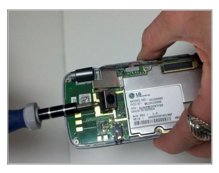
Remove the camera by carefully separating it from the tape underneath it.
