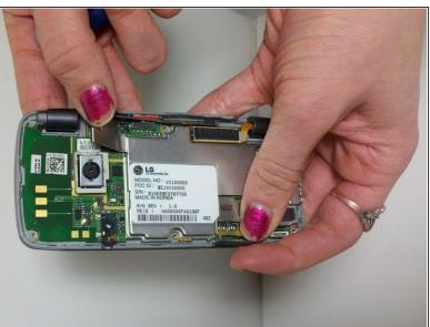
Slightly lift the small silver panel located to the right of the camera.
