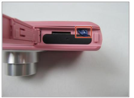
Locate the blue latch that holds the battery in the battery chamber.
