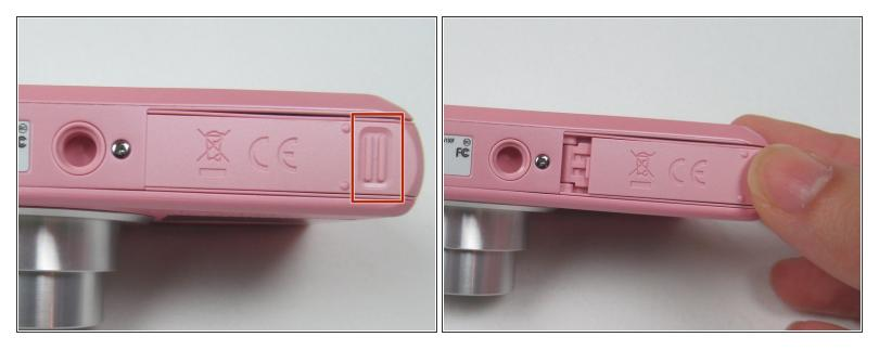
Locate the battery door and slide it to the right to unlatch it. Swing the battery door up to expose the battery chamber.
