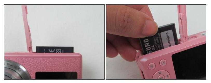
Once the latch is disengaged, the battery should pop up. Grab the battery and slide it up and out of the camera.
