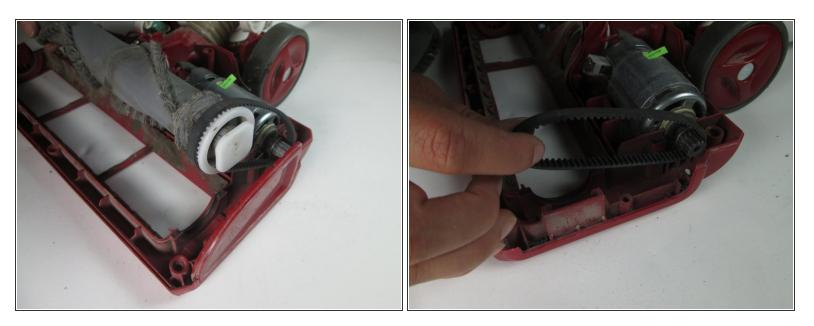
• Remove the roller belt from around the roller brush and the motor gear.
